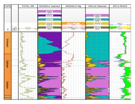
Figure 2 Comparison of standard ECS processing (WALK2) with advanced ECS acquisition and processing (MGWALK)
